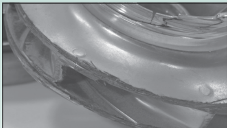
SAND-DAMAGED SUBMERSIBLE PUMP IMPELLER
