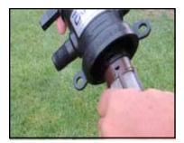
Pull the filter element straight off the housing. It should pull straight out.
