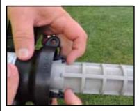
Using one hand for each clip might be the best method. This is easiest after the ilter has been installed. You might need to apply a little force to pull out the element as you lift the clips, since it may be stuck in place.
