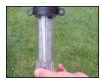
Hand tighten the clear bowl back into the housing.
